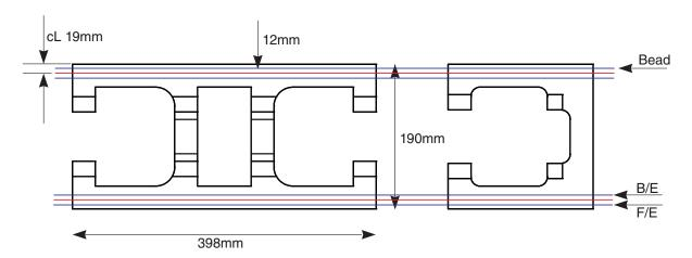
B/E = Back Edge of Expanded Bead F/E = Front Edge of Expanded Bead Bead = Centreline of Bead should be 19mm from outer edge on 190mm blocks
